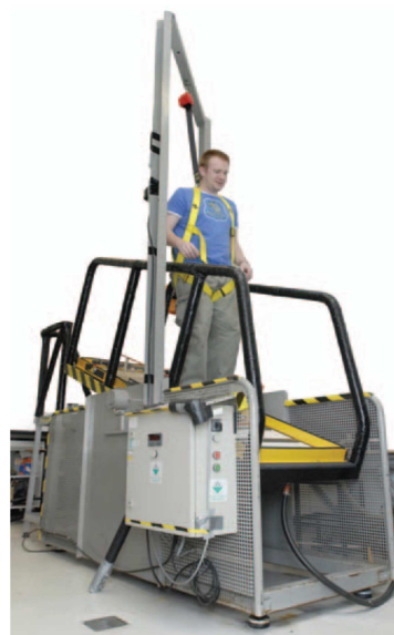
Fig. 3. The ramp friction coefficient test.
