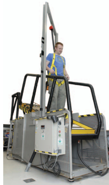
Figure 3. The ramp friction coefficient test
