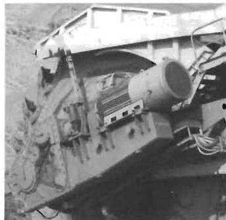
Fig. 2 Toothed gear transmission of BWE's working wheel
