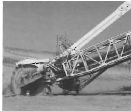
Fig. 1 The working wheel of a BWE
