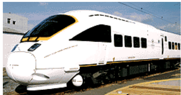
Figure 5 Express train built by Hitachi containing full-length friction stir welds of double-skin side and roof panels (welded from both sides) [2]
