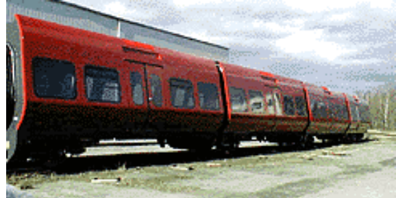
Figure 3 Alstom LHB trains for DSB Danish State Railways. FSWed roof panels for these trains are made at Hydro Marine Aluminium [2]
