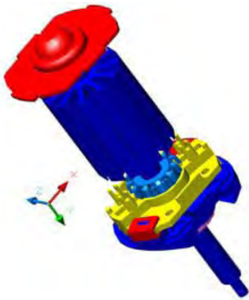
Fig.2. Electro motor, fan and thermostat
