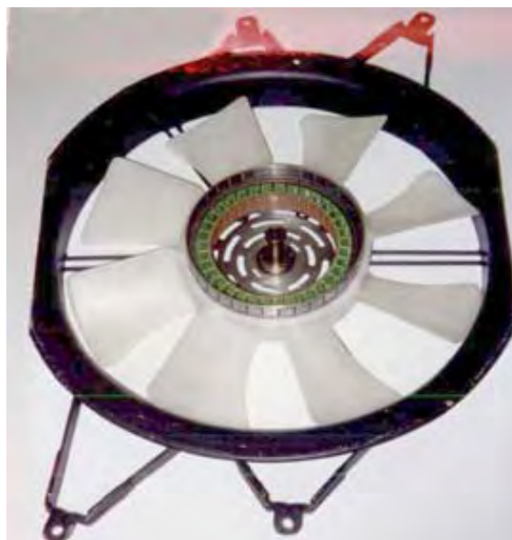
Fig. 4 a. Electro motor with rotor (rotor without collector and wire), circuit and electro motor
