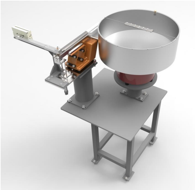
Fig. 1. The inner tube valve transfer unit as part of the machine for the inner tube assembly process.
