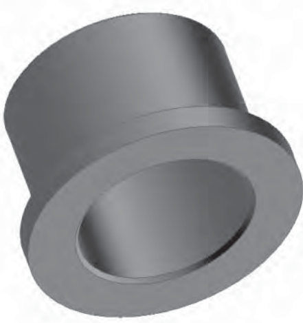
Fig. 12. 3D Model of Journal Bearing Casing Generated In Autodesk Inventor
